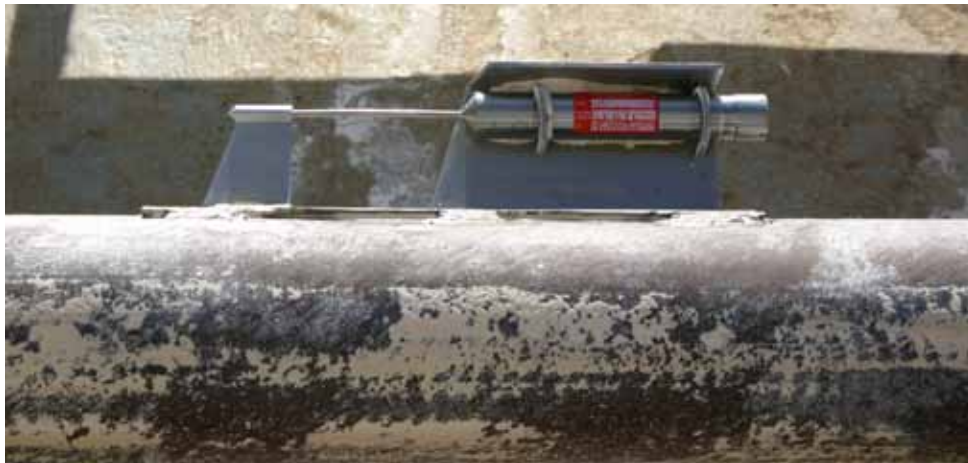
Figure 8. Arrangement for heat-flow measurements. Thermistors are attached at a set interval to the outside of the barrel of a 14 m –long gravity corer.
